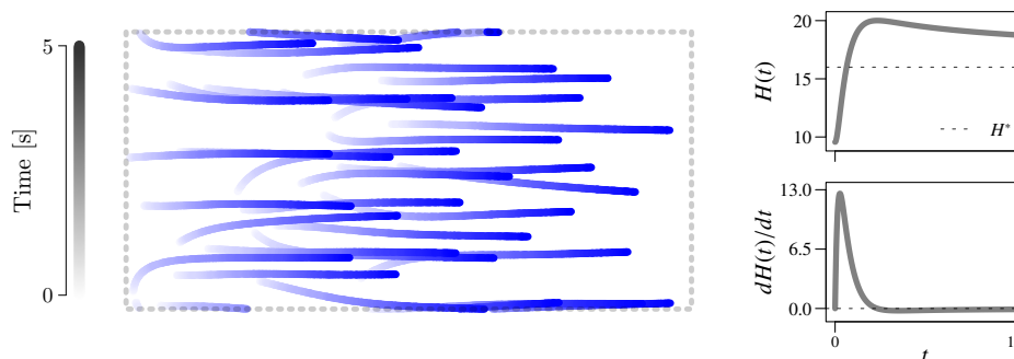
Figure 3. Simulation of a uni-direction flow used as a reference to compare the six numerical schemes Eqs (3.2)–(3.6), see Figure 4. Illustrative example of the leapfrog scheme (3.6) with \delta t = 0.001 \text{ s} .
