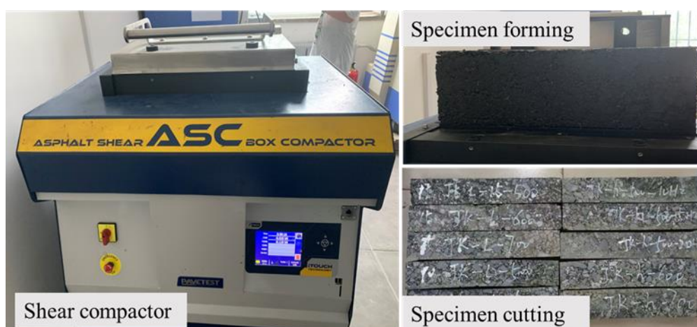
Figure 2. Forming and cutting of specimen.
