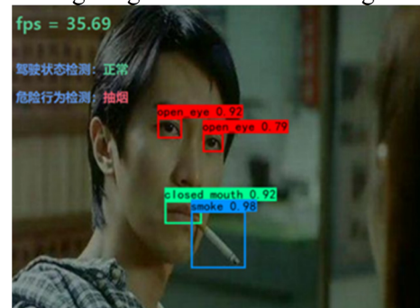
(d) The driving state is normal and the driving behavior is smoking
