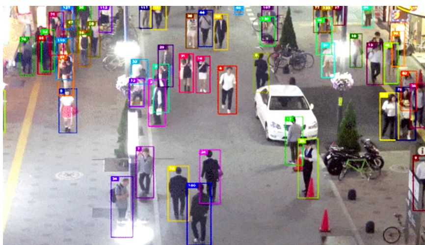
Figure 6. Multi person tracking with unique ID assignment using DeepSORT [65].
