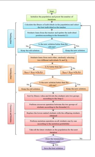
Figure 1. The flowchart of the ETLBO algorithm.
