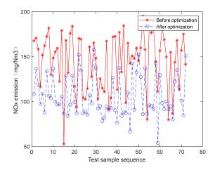
Figure 10. The comparison curve before and after the optimization of NO<sub>x</sub> emissions
