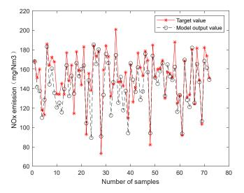
Figure 9. NO<sub>x</sub> emission testing model curve.
