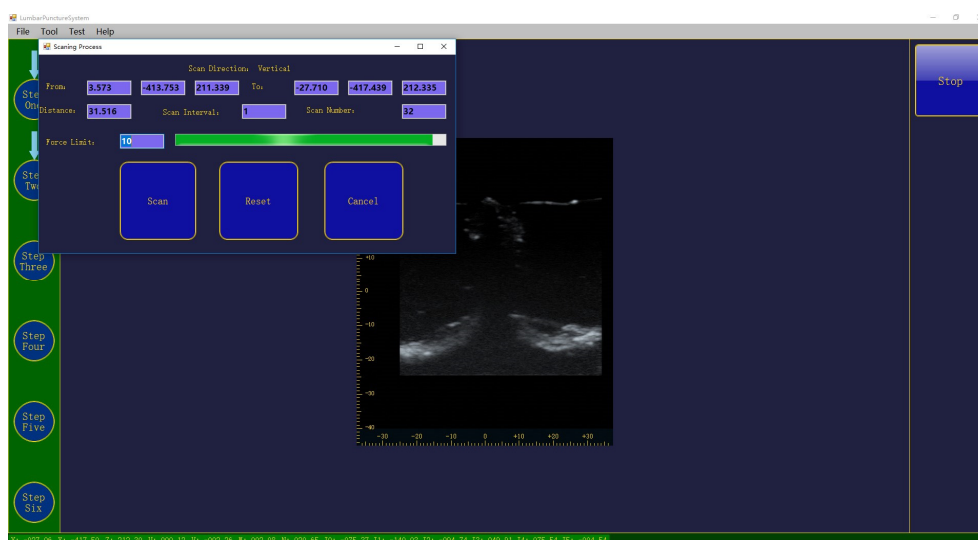
Figure 2. Two-dimensional ultrasound image acquisition program following robot arm scanning (the active green strip is the force status bar of probe).
