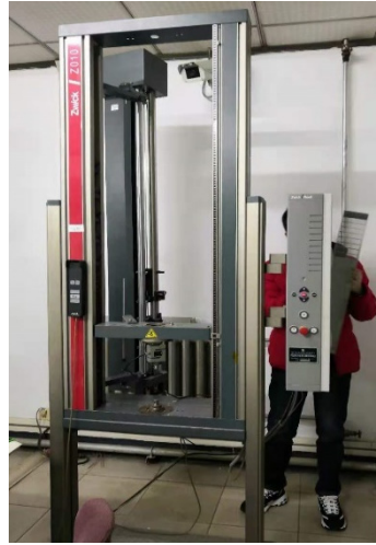
Figure 3. The Zwick Z010 material test device.
