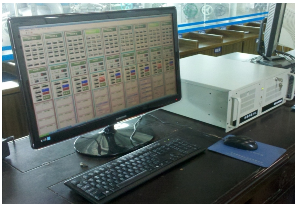
Figure 9. Optimal control experimental system of glucose feed rate in Chlortetracycline (CTC) fermentation process.
