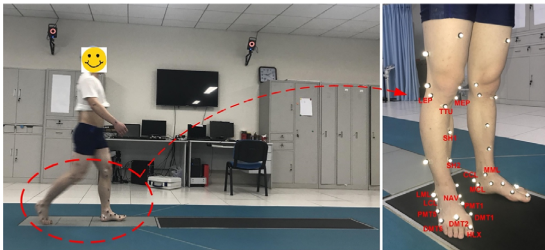
Figure 1. Tracking movements of subjects using a Vicon MX Motion Capture System. Markers are stuck on the shank and foot following the HFMM. LEP/MEP, lateral/medial epicondyle; TTU, tibial tuberosity; SH1/2, two points on the medial side of the tibia; LML/MML, lateral/medial malleolus; LCL/CCL/MCL, lateral/dorsal/medial calcaneus; NAV, navicular; PMT1/PMT5, proximal end of the first and fifth metatarsals; DMT1/2/5, distal end of the first/second/fifth metatarsals; HLX, hallux.
