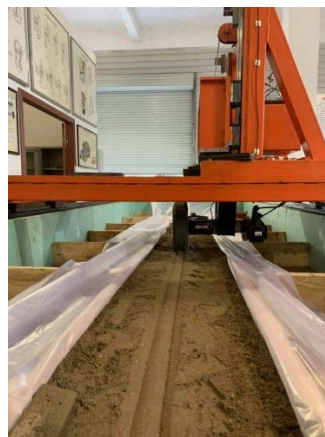
Figure 12. The tire indentation formed during the test.
