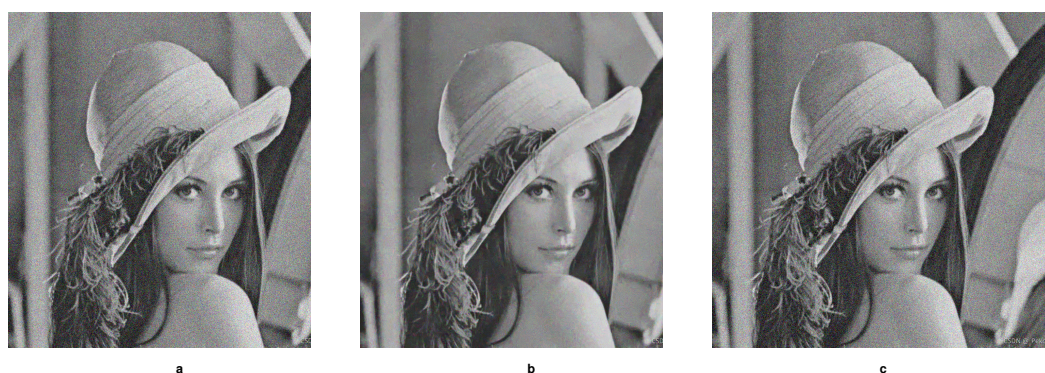
Figure 9. Grayscale image denoising enhancement: (a) Gaussian noisy ( \sigma = 0.02 ); (b) BM3D; (c) MRNNs with control strategy (3.10).
