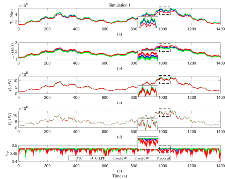
Figure 9. Simulation 1: (a) generator torque T_e , (b) rotor speed \omega_m , (c) generator power P_e , (d) aerodynamic power P_a , (e) power coefficient C_p .
