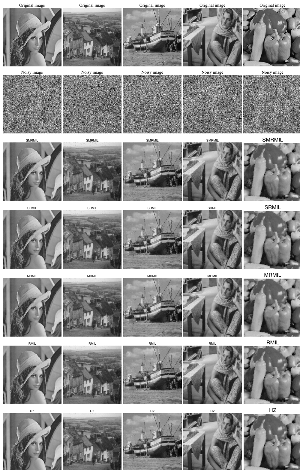
Figure 10. Image denoising under the standard Armijo line search. Row 1: Original images; Row 2: Noisy images (salt-and-pepper noise ratio is 0.8); Rows 3–7: Restored images by the SMRMIL, SRMIL, MRMIL, RMIL, and HZ methods, respectively.
