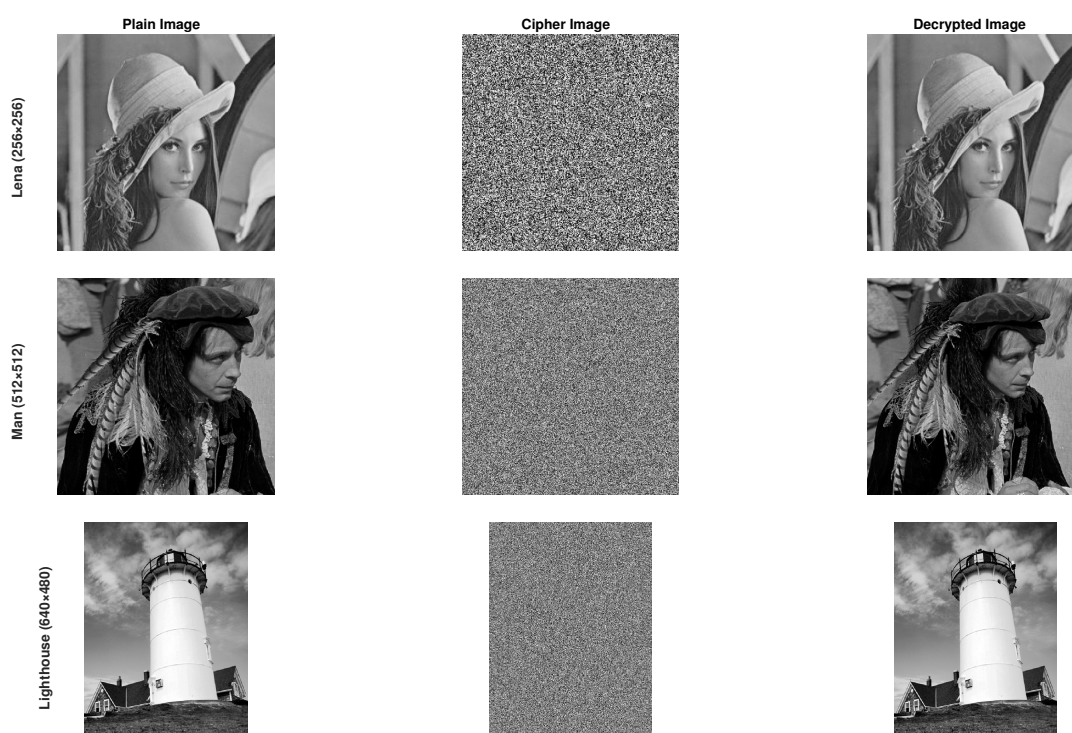
Figure 6. Combined encryption-decryption results on three grayscale images with different resolutions. Rows correspond to (a) Lena ( 256 \times 256 ), (b) Man ( 512 \times 512 ), and (c) Lighthouse ( 640 \times 480 ). Columns show the plaintext, ciphertext, and decrypted image, respectively.
