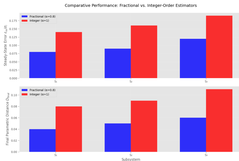
Figure 6. Comparative performance: (top) Steady-state error \varepsilon_{ss} ; (bottom) parametric distance D_{final} for fractional ( \alpha = 0.8 ) and integer-order ( \alpha = 1 ) estimators.
