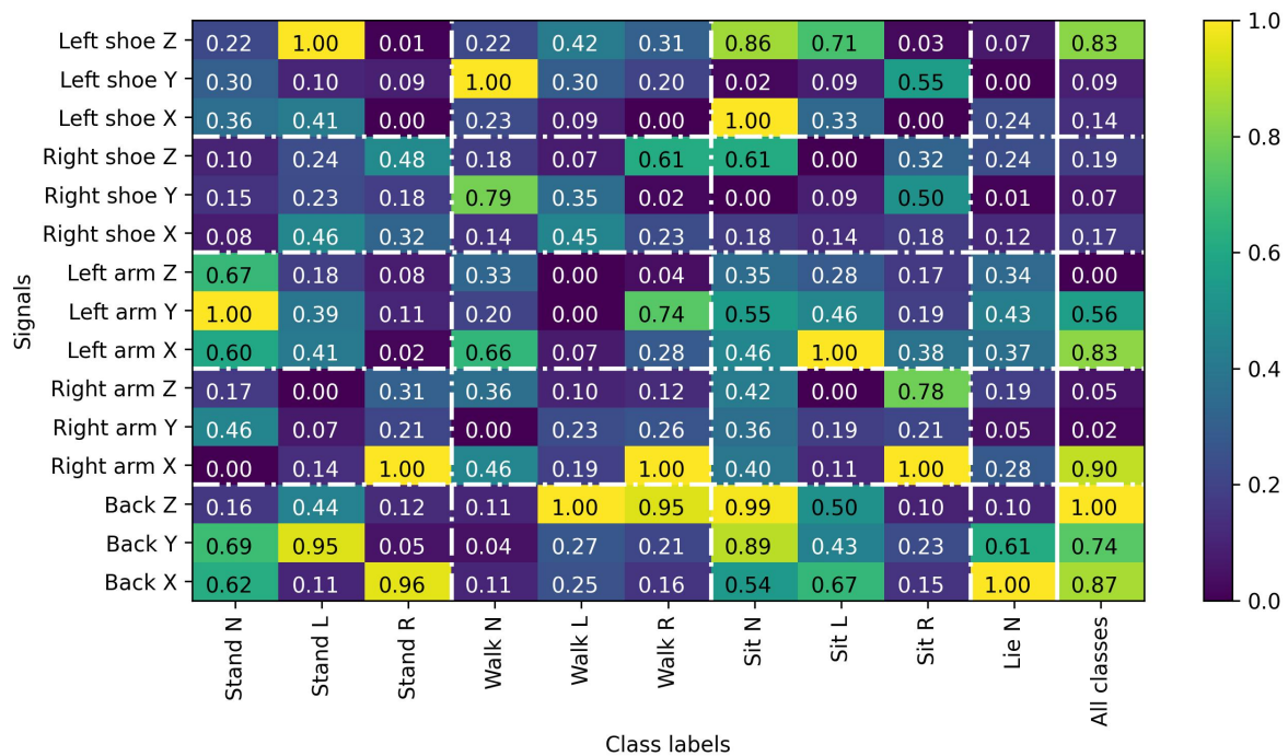
Figure 4. Example of signals importance to all classes expressed by SIM I_{\text{mat}}(\mathbf{X}) and SIV I_{\text{vec}}(\mathbf{X}) calculated to CNNs of Condition A described in Section 5. Columns 1 to 10 are SIM and column 11 is SIV (“All classes”). The values are standardized from zero to one in each column. The greater the cell’s value, the greater is the relevance of signal s on estimation class c' .
