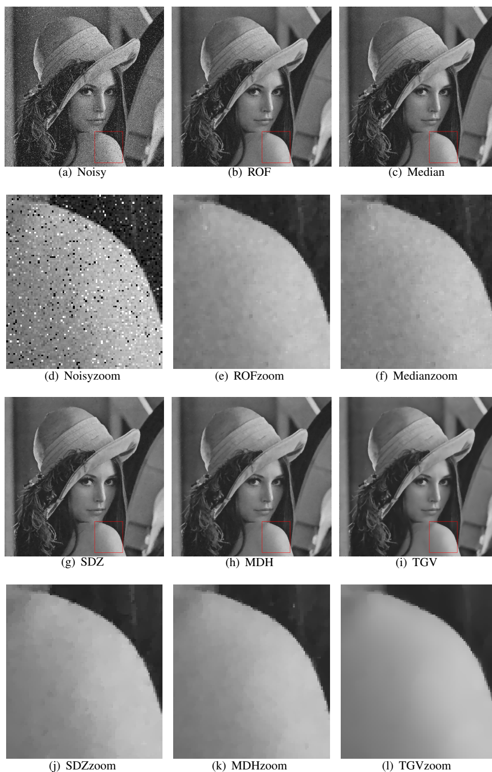
Figure 3. The noisy image, restored images and the locally zoomed images, respectively. For ROF method, \lambda = 2.6 . For SDZ method, \eta = 0.68, \lambda = 5.2 . For MDH method, \lambda = 45 . For the proposed method, \lambda = 22, \tau = 0.65 .
