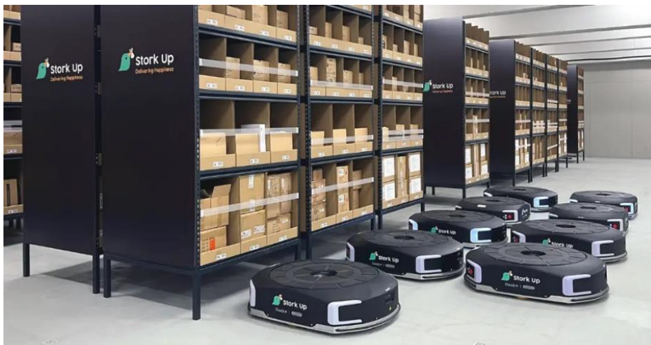
Figure 1. Robotic mobile fulfillment system.
