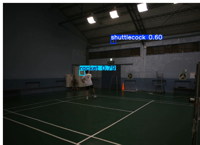
Figure 3. Result of YOLO-based racket and shuttlecock detection.
