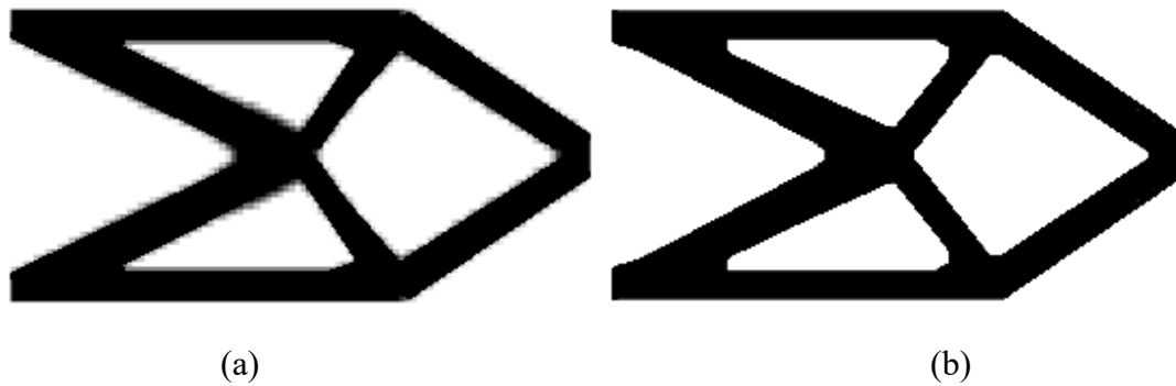
Figure 13. Obtained optimal topological structures of cantilever beam by using two methods: (a) represents obtained optimal topological structure by using the existing SIMP scheme based on B-spline; (b) represents obtained optimal topological structure by using the proposed method.
