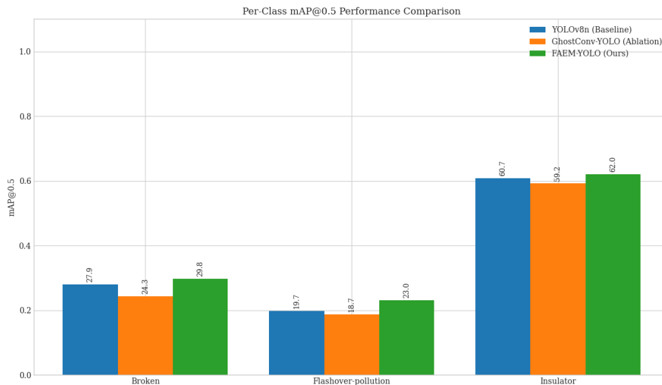
Figure 16. Per-class mAP@0.5: FAEM-YOLO beats YOLOv8n and GhostConv across all classes, with biggest gains on Broken and Flashover-pollution.
