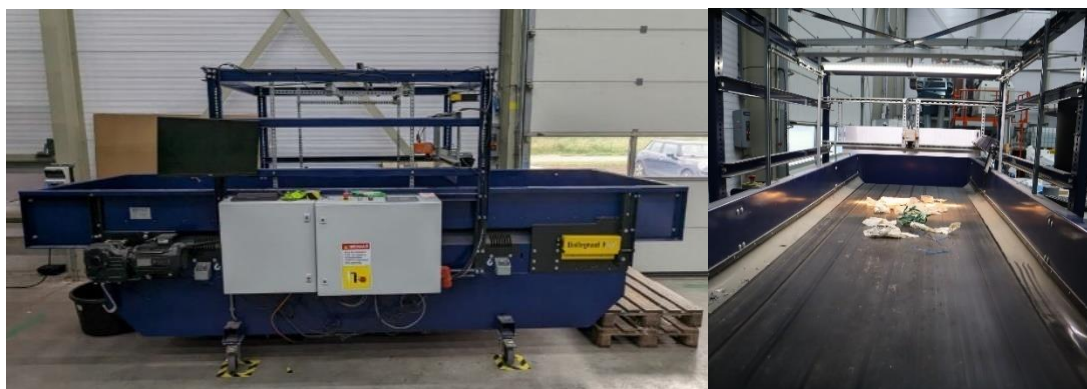
Figure 1. Photographs of the actual data collection platform used, integrating Specim FX 17 camera and the halogen light source used for data collection (left); Actual plastic waste samples on the conveyor belt (right).
