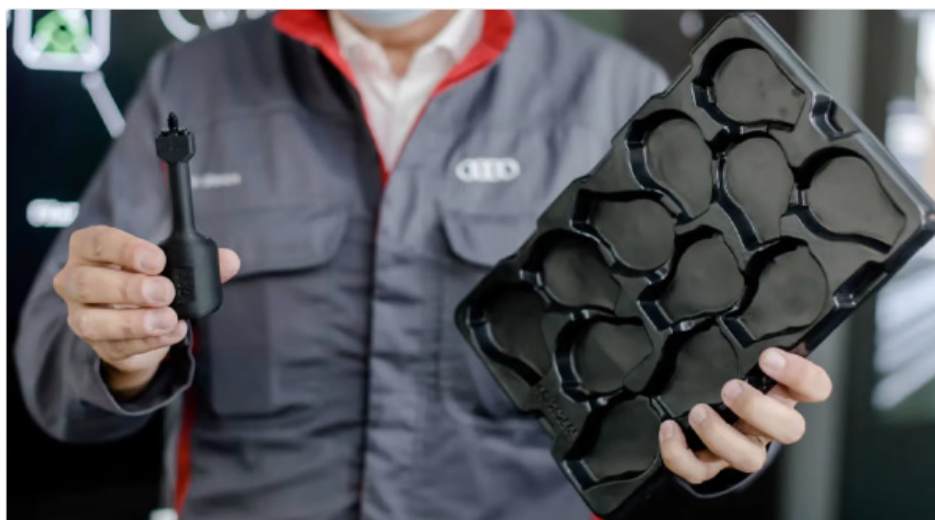
Figure 24. A technician at Audi holds up a manufacturing tool and the plastic packing waste it was 3D printed from [83].
