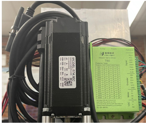
Figure 9. Closed loop servo motor with encoder and drivers.
