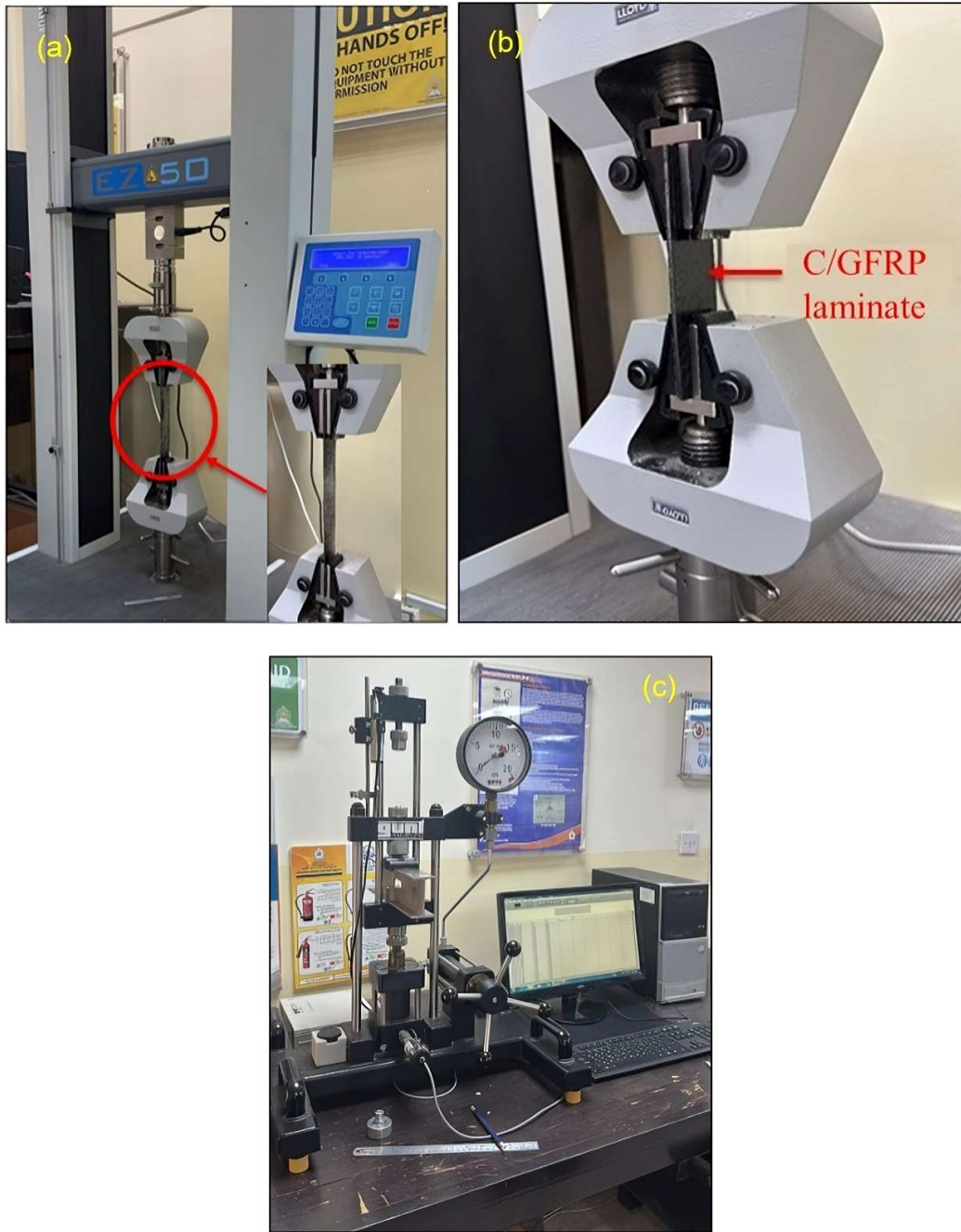
Figure 2. Experimental set up for the (a) tensile test, (b) compression test, and (c) flexural test.
