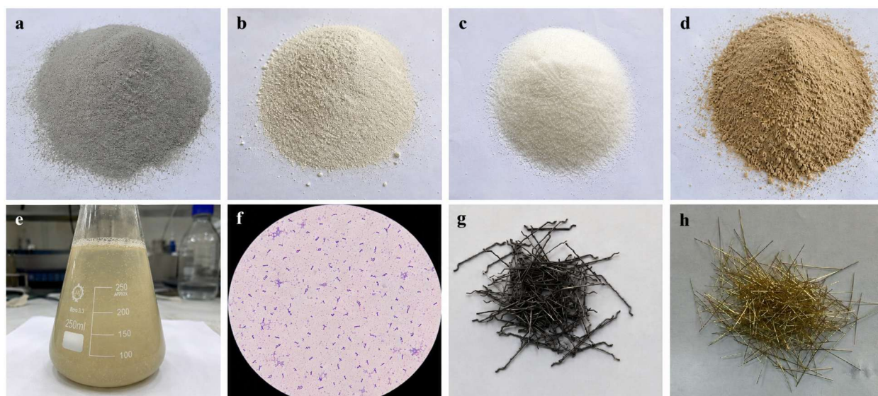
Figure 2. Ingredients involved in the formation of geopolymer SIFCON: (a) RHA, (b) nanobentonite, (c) PAM, (d) Bacillus subtilis bacteria, (e) Bacillus subtilis bacterial solution, (f) microscopy picture of Bacillus subtilis bacteria, (g) hooked-end steel fibers, and (h) straight steel fibers.
