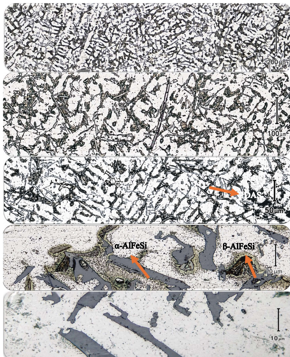
Figure 4. Microstructure of Keller's etchant at different magnifications.
