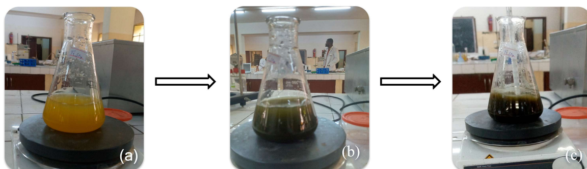
Figure 3. Synthesis of \text{Fe}_2\text{O}_3 NPs in solution from extracts of A. alboviolaceum leaves.
