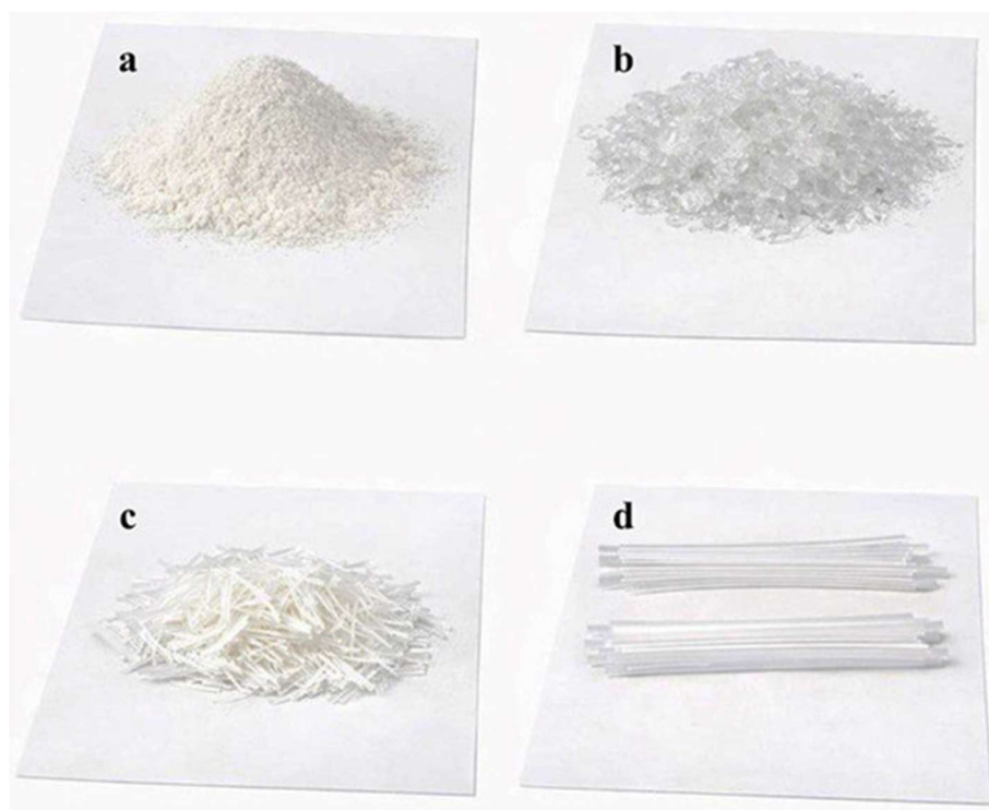
Figure 1. Materials used in this study, including: (a) metakaolin; (b) crushed recycled glass; (c) ARGF; and (d) both coated and uncoated optical glass fibers.
