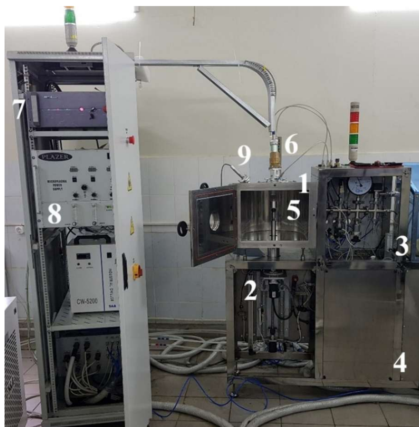
Figure 2. External view of the technological complex and vacuum chamber with a rotary manipulator for welding in a protective controlled atmosphere at various pressures.
