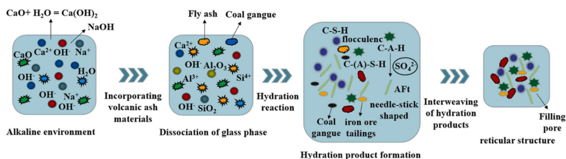
Figure. 4. Alkali-excited ceramsite hydration mechanism diagram (Reproduced from Ref. [19] with permission).
