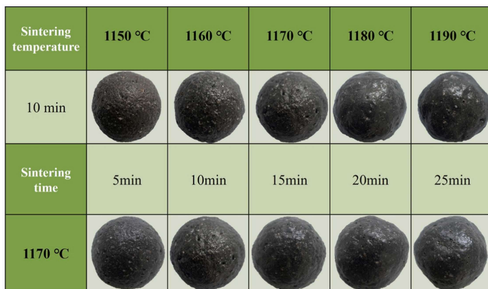
Figure 3. Effect of the sintering temperature and duration on the surface morphology of ceramsite (Reproduced from Ref. [69] with permission).
