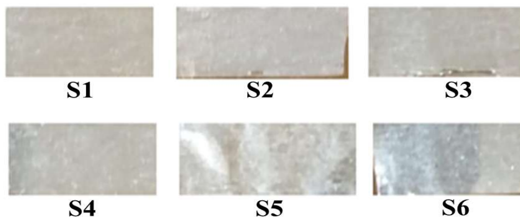
Figure 2. Suitable shape of synthesis shielding alloys using the melt-spun process.
