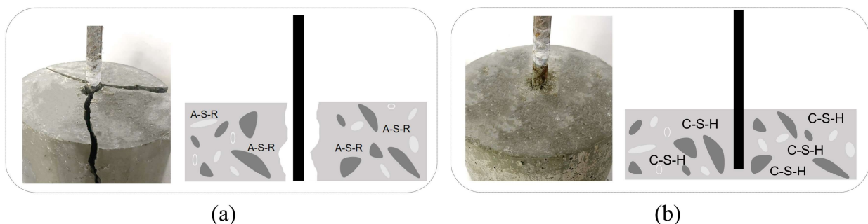
Figure 7. Failure modes of specimens: (a) splitting failure; (b) pull-out damage.
