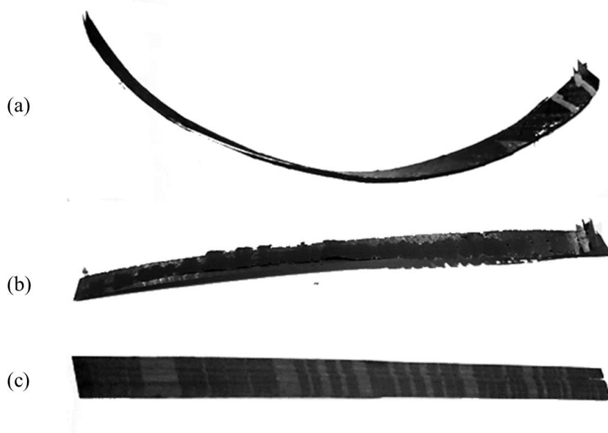
Figure 3. Scrap tapes for the different panel lay-ups: (a) [0,+45,90,-45]_{2s} panel; (b) [0,90]_{4s} panel; (c) [0]_{16} panel.
