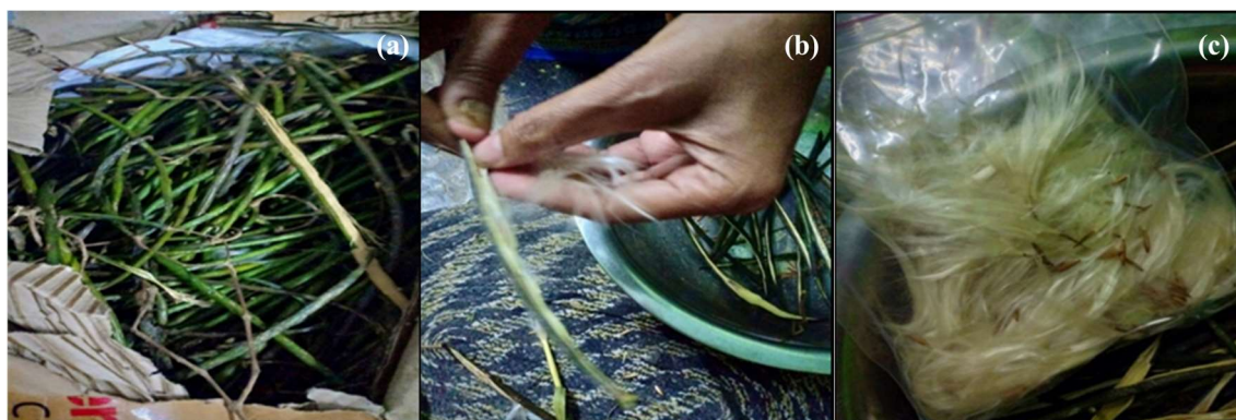
Figure 3. (a) WTSFs seedpods (b) Extraction of WTSFs from seed pods, (C) Fibers stored in Polythene bags.
