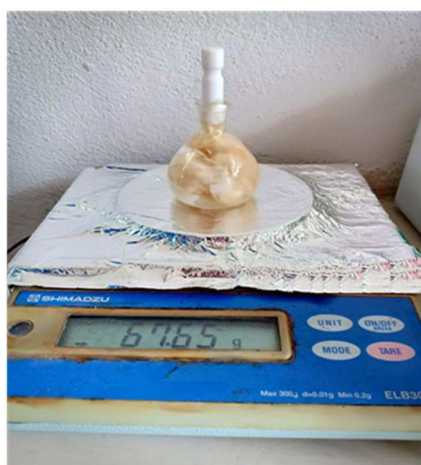
Figure 7. Density determination of WTSFs fibers.
