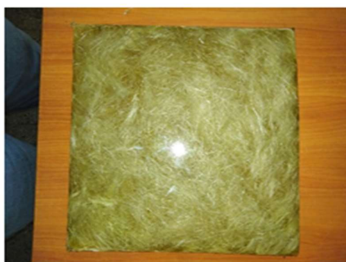
Figure 1. Image of hybrid sisal-cotton fiber reinforced polyester composite during fabrication.
