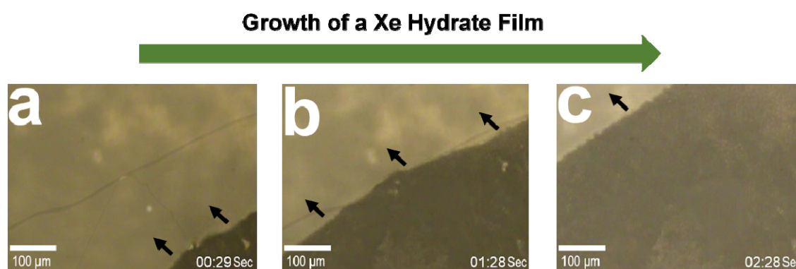
Figure 3. Chronological illustrations depicting the lateral growth of a Xe hydrate film on mica following a cooling cycle at 263.13 K under 2.75 bar of Xe at growth time: (a) t = 0:29 s, (b) t = 1:28 s, and (c) t = 2:28 s.
