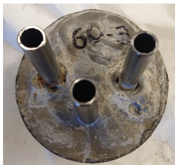
Figure 1. Cement sample with inserted electrodes, top view. The reference pipe is closest to the viewer.
