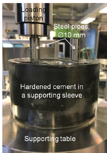
Figure 3. Setup for a push-out test performed on a cemented electrode.
