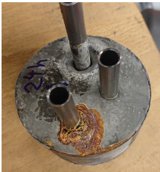
Figure 7. Corrosion at the positive electrode after 24 h of electric field application (4 V).
