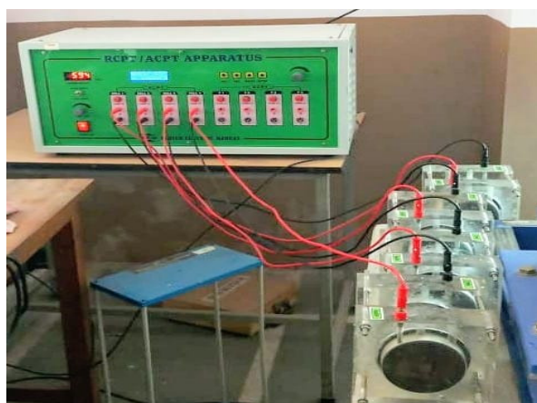
Figure 1. Rapid Chloride Permeability Test set-up.
