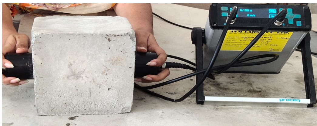
Figure 2. UPV test setup.
