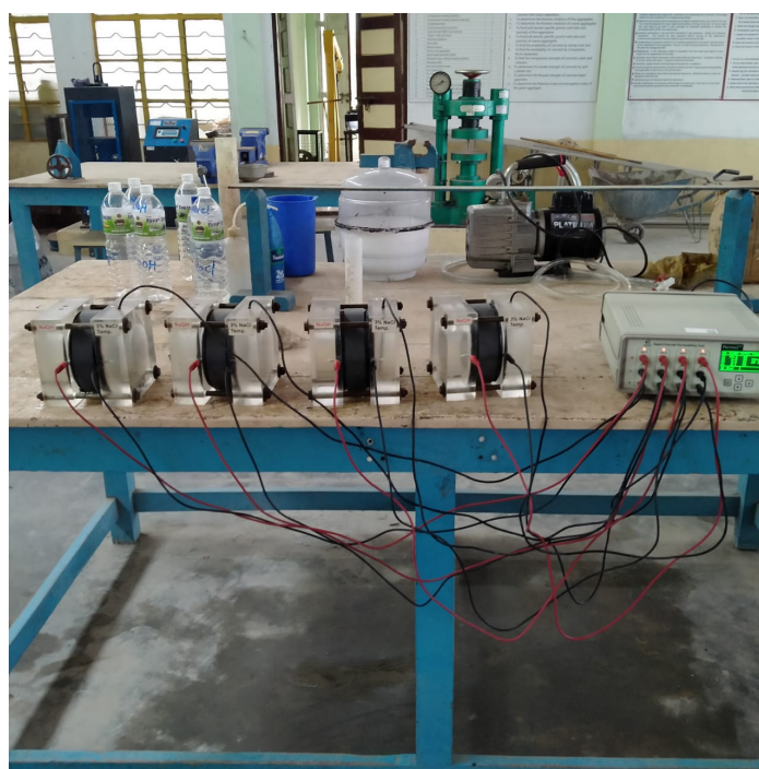
Figure 3. Setup for rapid chloride penetration test.
