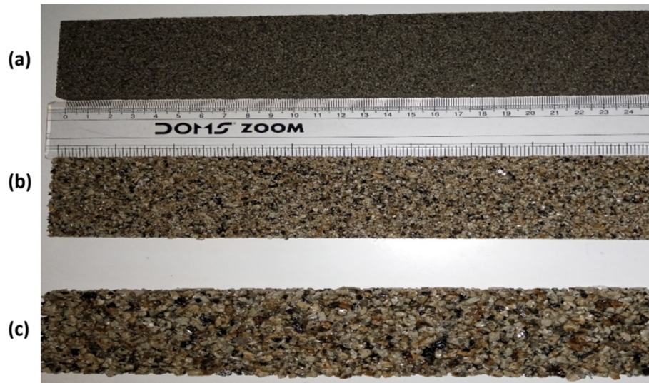
Figure 6. Flexural test specimens: (a) fine, (b) medium, (c) coarse particles.
