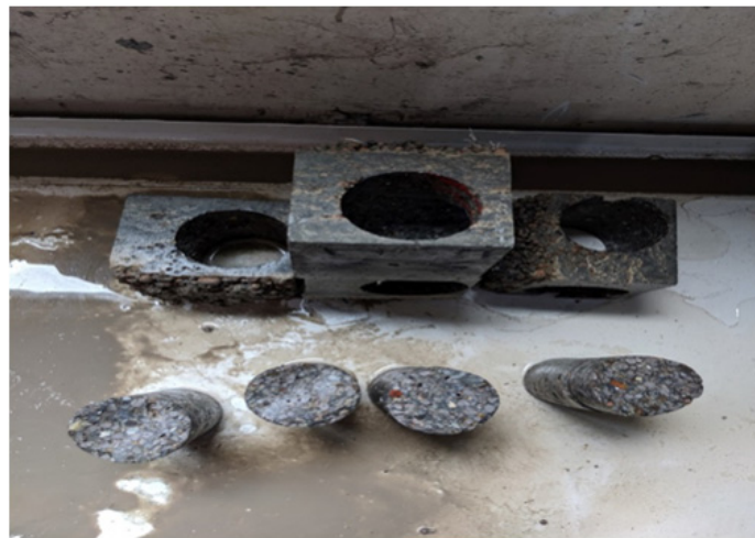
Figure 2. Concrete samples is cored and sliced for Heat Flow test.
