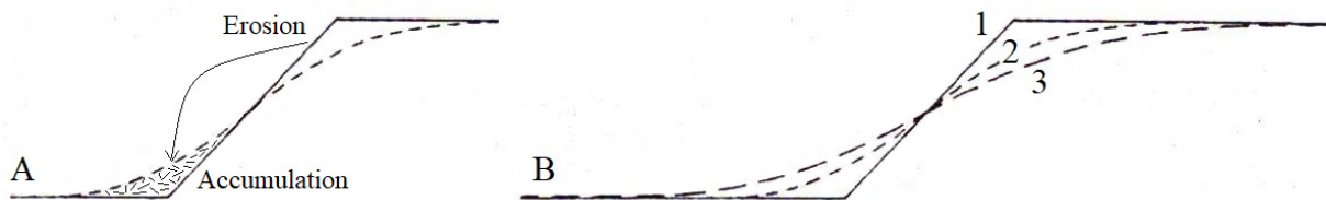
Figure 6. A) Schematic model for colluvial wedge development at the slope foot after upslope failure. B) Schematic steps of slope retreat [24].
