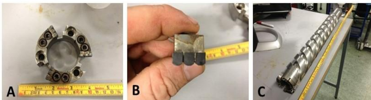
Figure 3. SINTEF-modified CRREL coring auger used for permafrost: (A) drill crown; (B) PCD inserts; (C) assembled corer.
