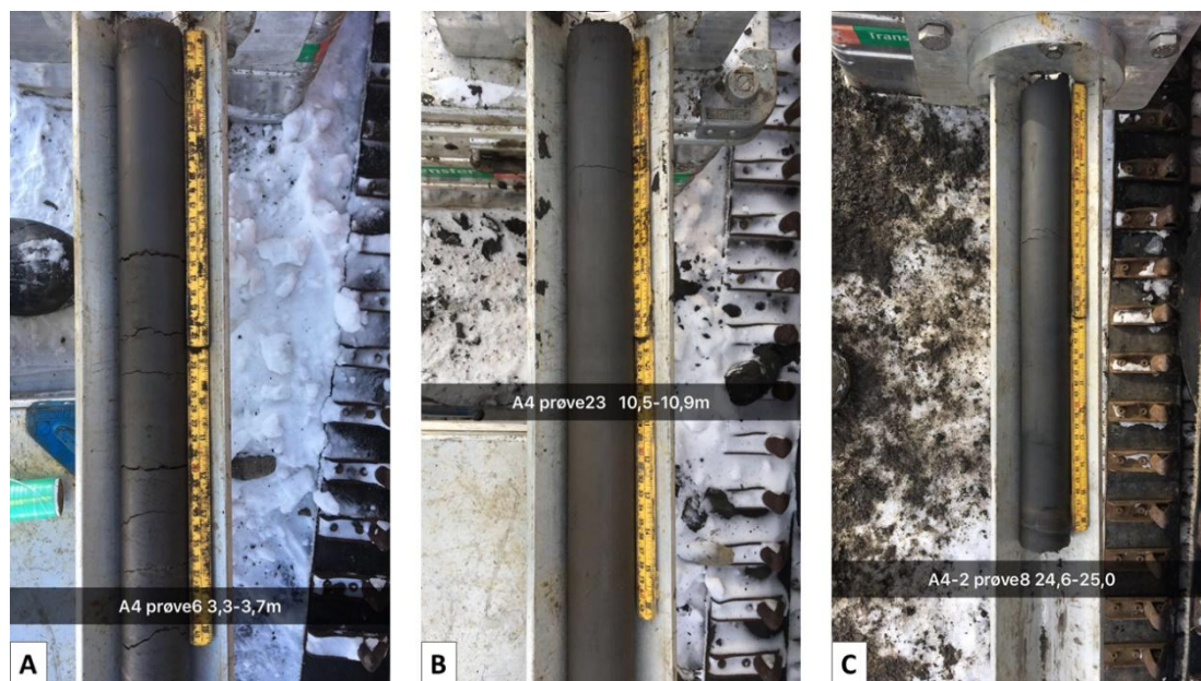
Figure 5. Core samples from borehole A4. Depths: (A) 3.3–3.7 m; (B) 10.5–10.9 m; (C) 24.6–25 m.
