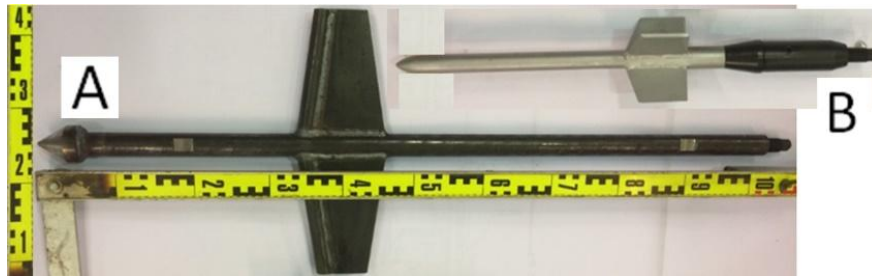
Figure 4. Column (A, “PK2/100”) and vane penetrometer (B, “PS130/65”) for columns. A: Tip underside area = 100 cm 2 and width –375 mm. B: Width –130 mm and height –65 mm [58].
