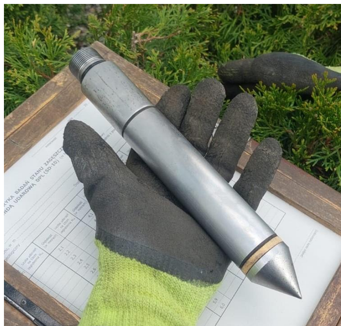
Figure 4. Used, partially worn penetrometer (b) prepared for testing.
