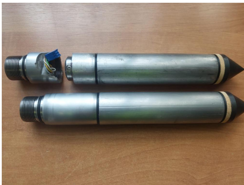
Figure 1. Two cones, with which more than 1000 m of soundings were performed. On top, a cone that suffered typical damage during sounding after one year of use.
