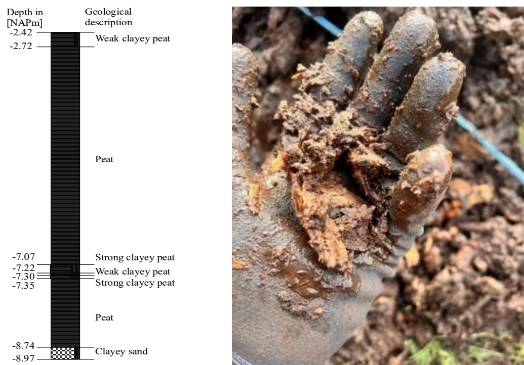
Figure 2. (a) Typical borehole log (b) wood remnants from peat at 1 m depth below the surface.
