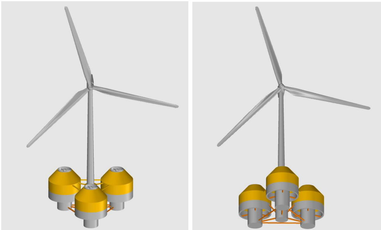
Figure 6. The examined REFOS multi-purpose floating structure.
