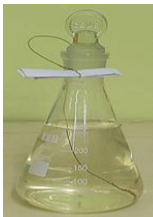
The etching solution with Normality of 6.25N
