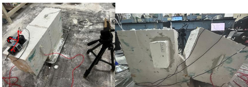
Figure 5. Instability process of a rock mass model.
