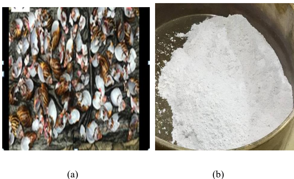
Figure 2. (a) Dried snail shells and (b) calcined and ground snail shell powder.
